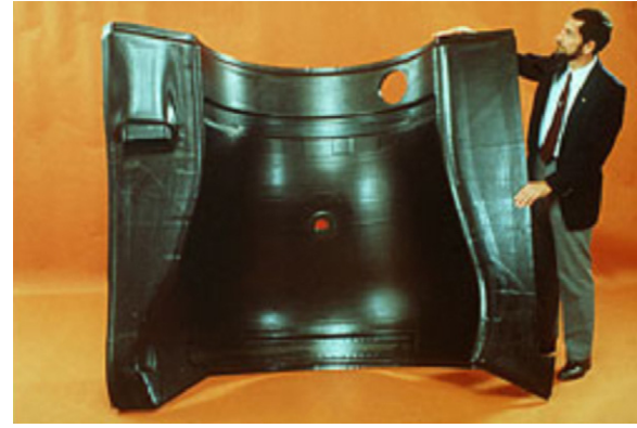
Fig. 9. A typical tool used to repair core cowl composite layers ( http://www.aerostructures.goodrich.com/html/rd_nonmetals.asp ).
