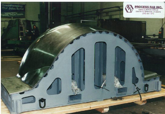
Fig. 8. An example core cowl lay-off tool ( http://www.processfab.com/imx/part11.jpg ).
